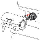
4. Adjust position and lock nut
