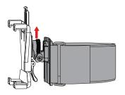
4. Rotate the nut to adjust up and down
