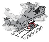
5. Rotate the nut to adjust left and right
